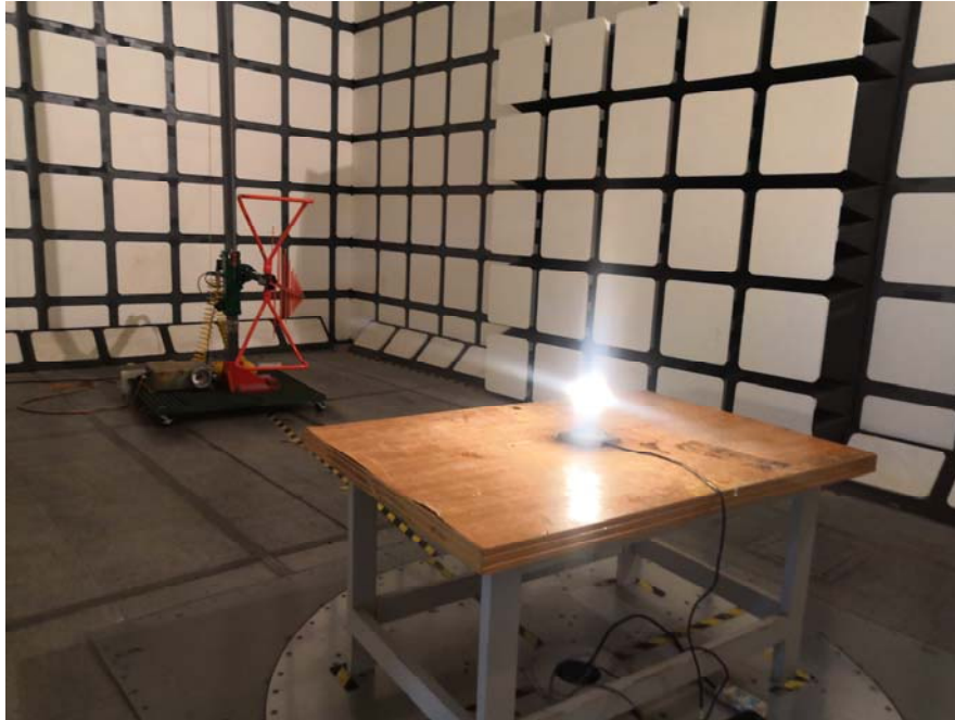
Radiated Emissions View (Below 1 GHz)
