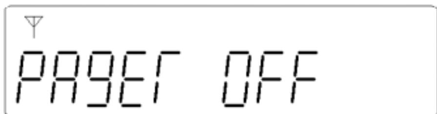
Press the Read Button ( ) to turn off. “OFF” and current time will display at the same time on the Screen to confirm the pager is in off mode. Clock is working While pager in off mode.
