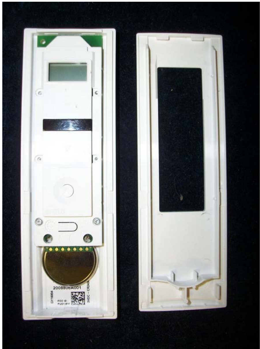
Figure 7.3 Inside View (5 Channel, 2008806)
