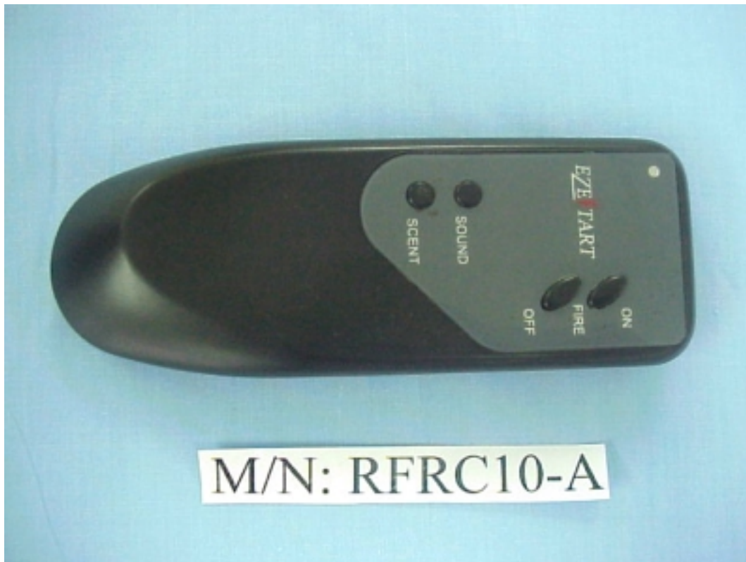
FIGURE 3 RADIO REMOTE CONTROLLER (M/N: RFRC10-A) GENERAL APPEARANCE (FRONT SIDE)
