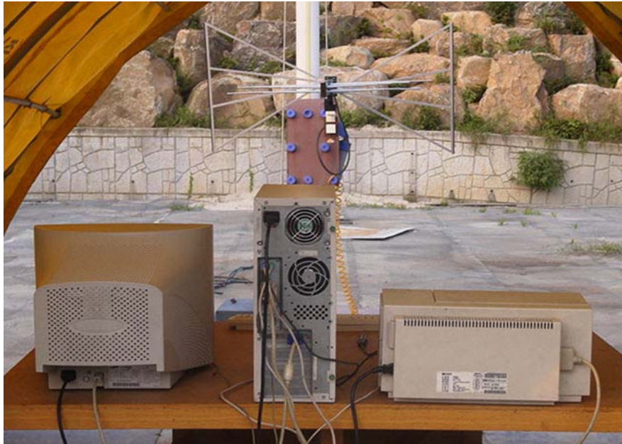
Photograph 1 : Setup for radiated Emissions
