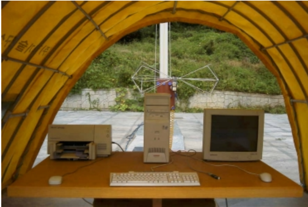
Photograph 1 : Setup for radiated Emissions
