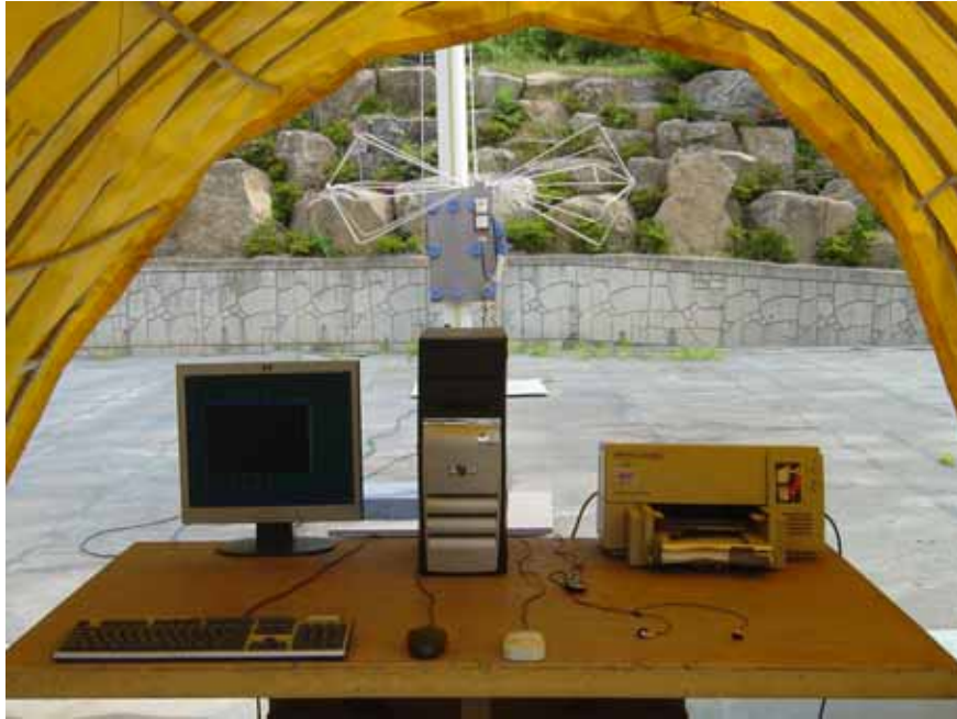
Photograph 1 : Setup for radiated Emissions
