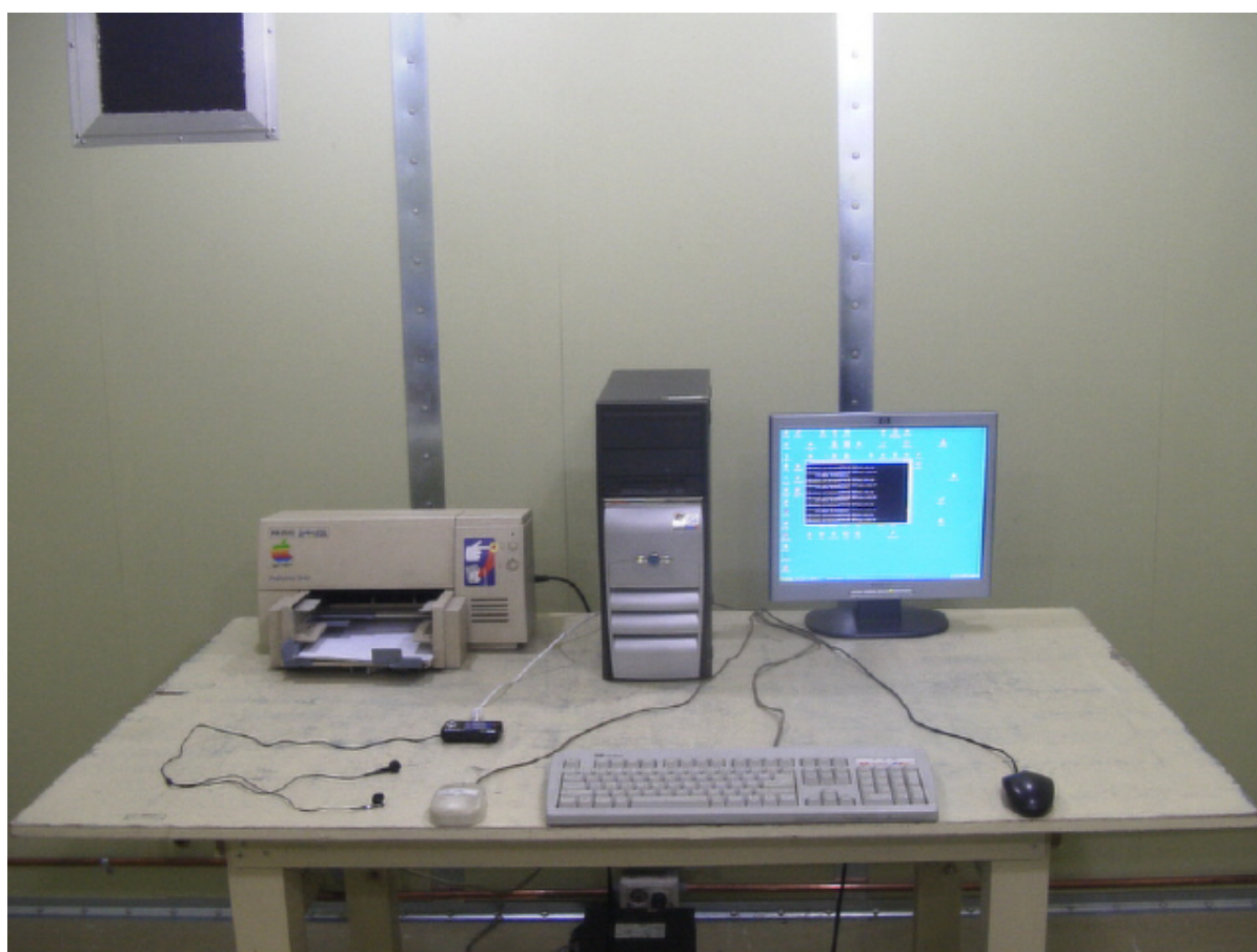
Photograph 2 : Setup for Conducted Emissions
