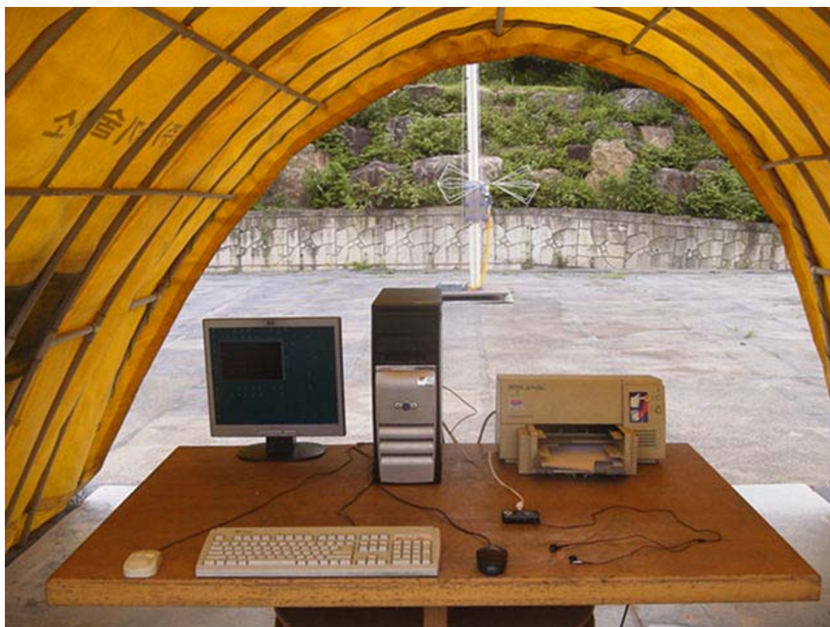
Photograph 1 : Setup for radiated Emissions
