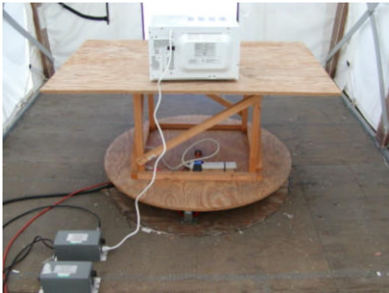
**Radiated Setup Photograph – Front View**
