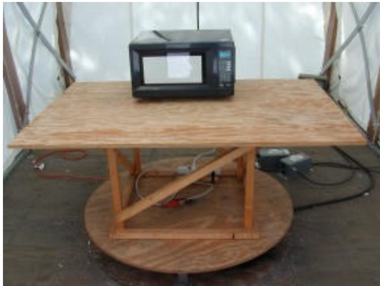
**Radiated Setup Photograph – Rear View**
