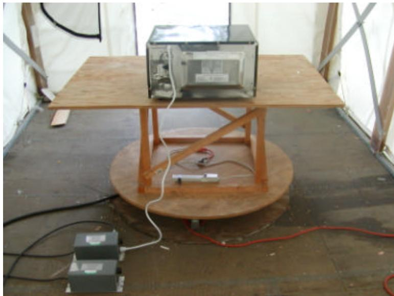
**Radiated Setup Photograph – Front View**
