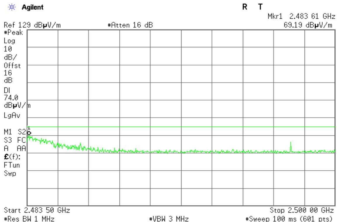
**Detector mode: Average****Polarity: Horizontal**
