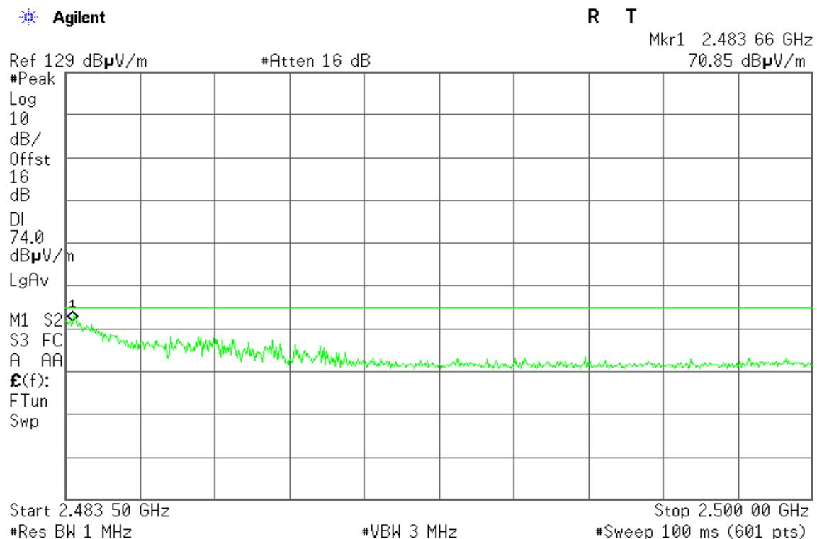
**Detector mode: Average****Polarity: Horizontal**
