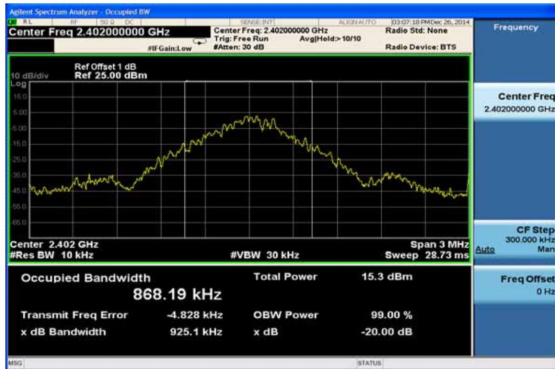
**20dB Bandwidth Test Data CH-Mid**
