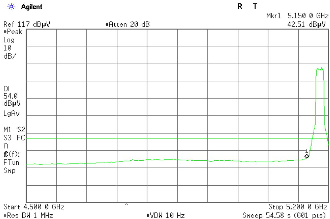
**Band Edges (IEEE 802.11a mode / 5320 MHz)****Detector mode: Peak****Polarity: Vertical**
