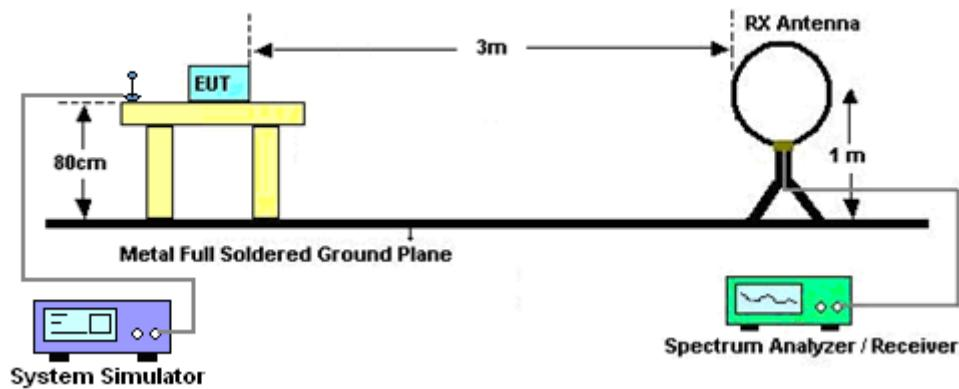
For radiated test from 30MHz to 1GHz
