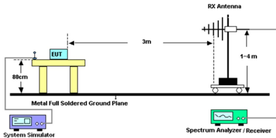
**For radiated test above 1GHz**
