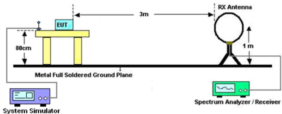
For radiated test from 30MHz to 1GHz
