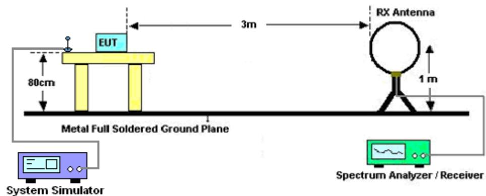
For radiated test from 30MHz to 1GHz
