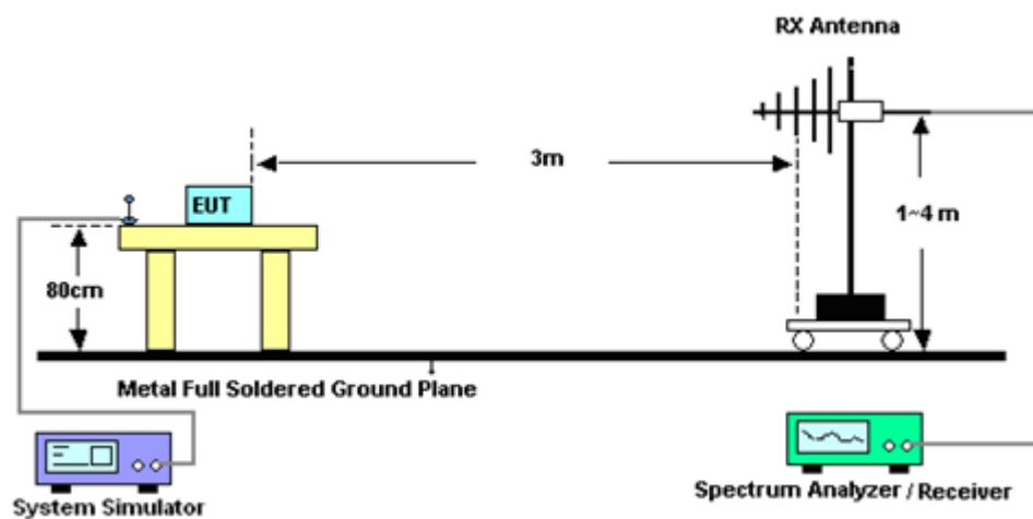
**For radiated test above 1GHz**
