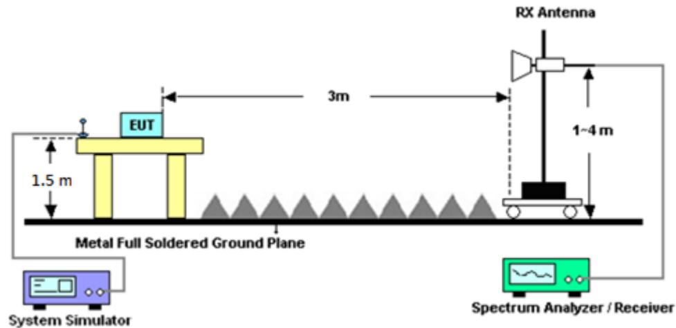
**3.1.4 Test Result of Field Strength of Spurious Radiated**
