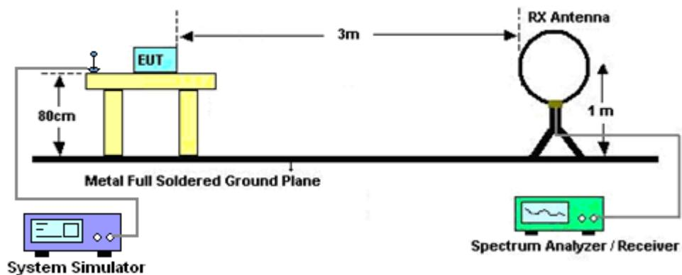
For radiated test from 30MHz to 1GHz
