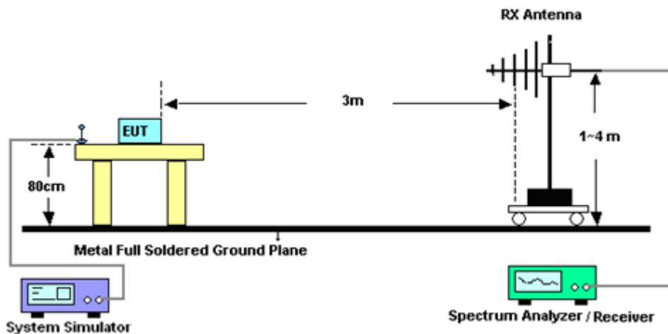
**For radiated test above 1GHz**
