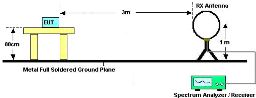
For radiated emissions from 30MHz to 1GHz
