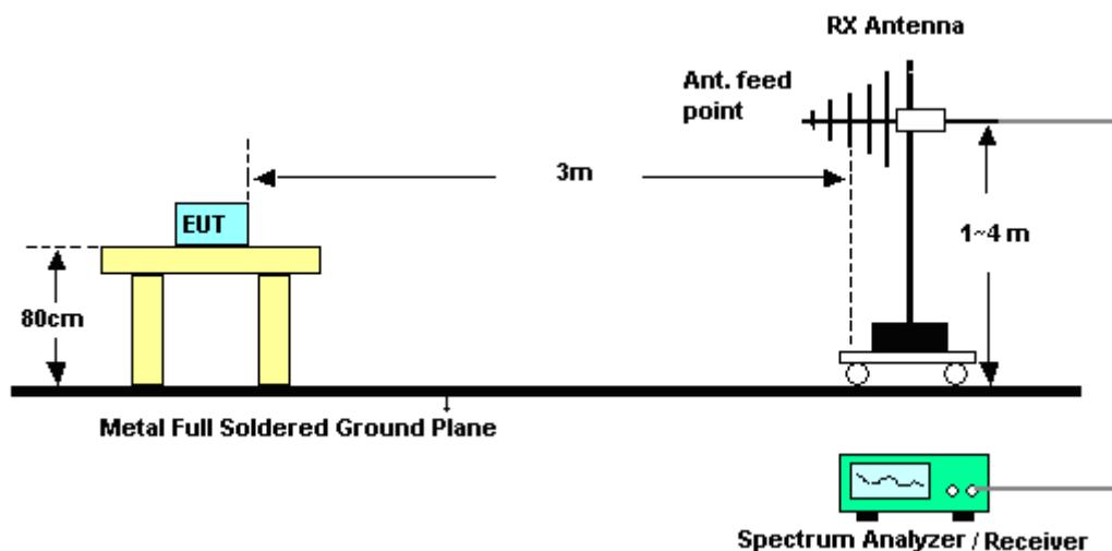
**For radiated emissions above 1GHz**
