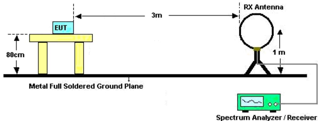
For radiated emissions from 30MHz to 1GHz
