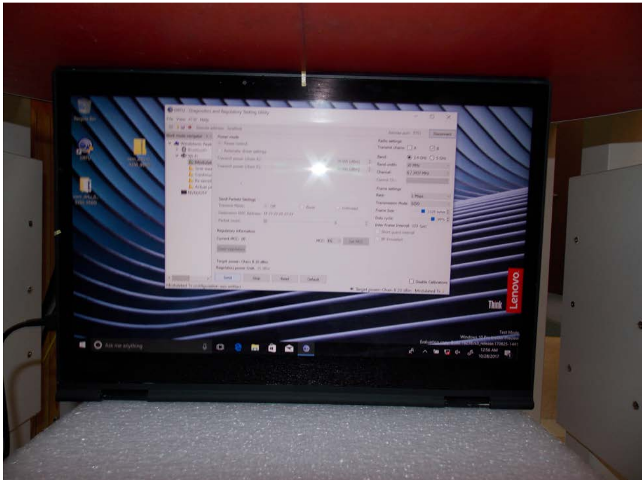
Test Position Top (Same for Both) 0 mm Gap
