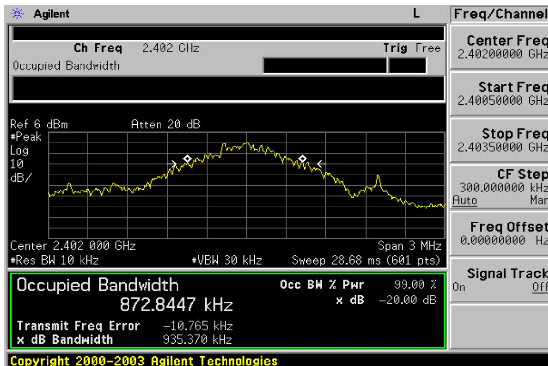
**20dB Band Width Test Data CH-Mid**
