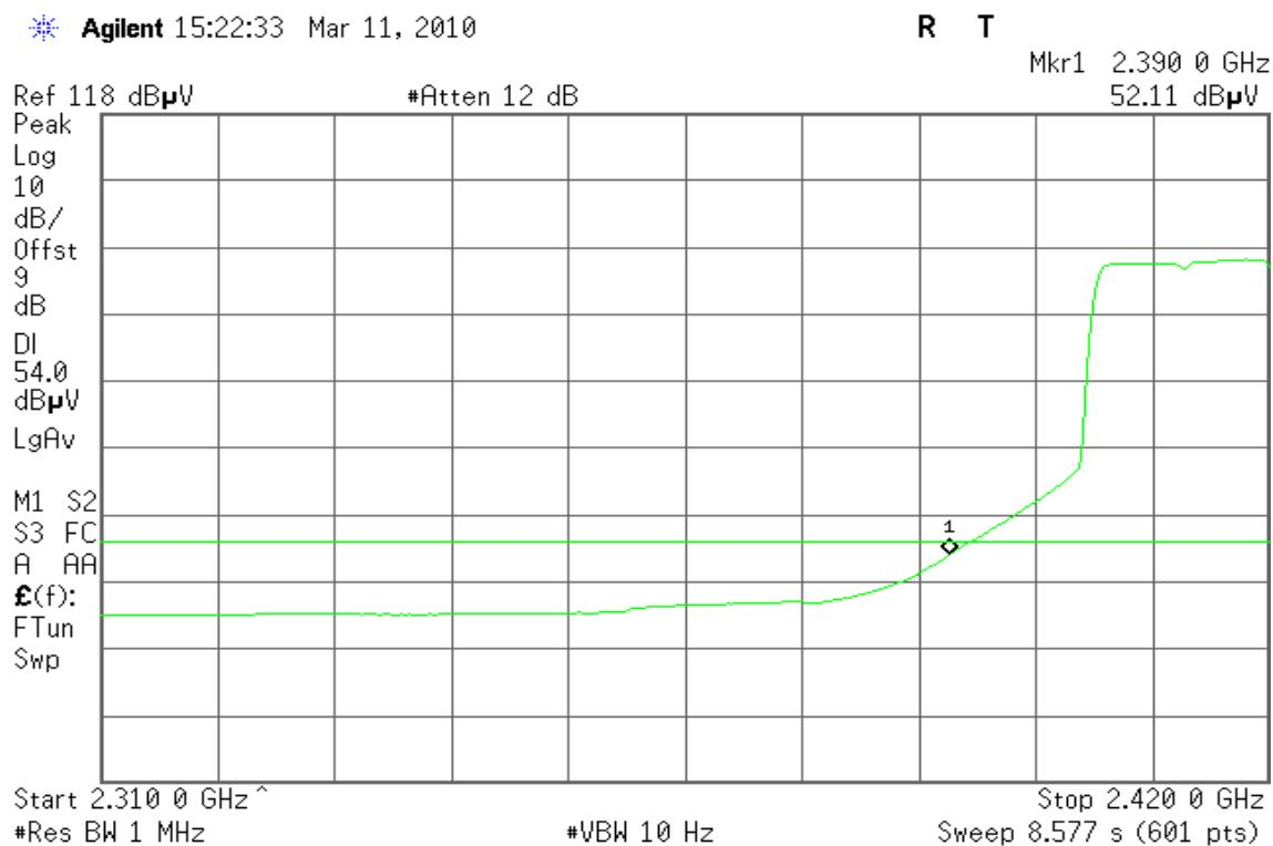
**Band Edges (IEEE 802.11g mode / CH High)****Detector mode: Peak****Polarity: Vertical**
