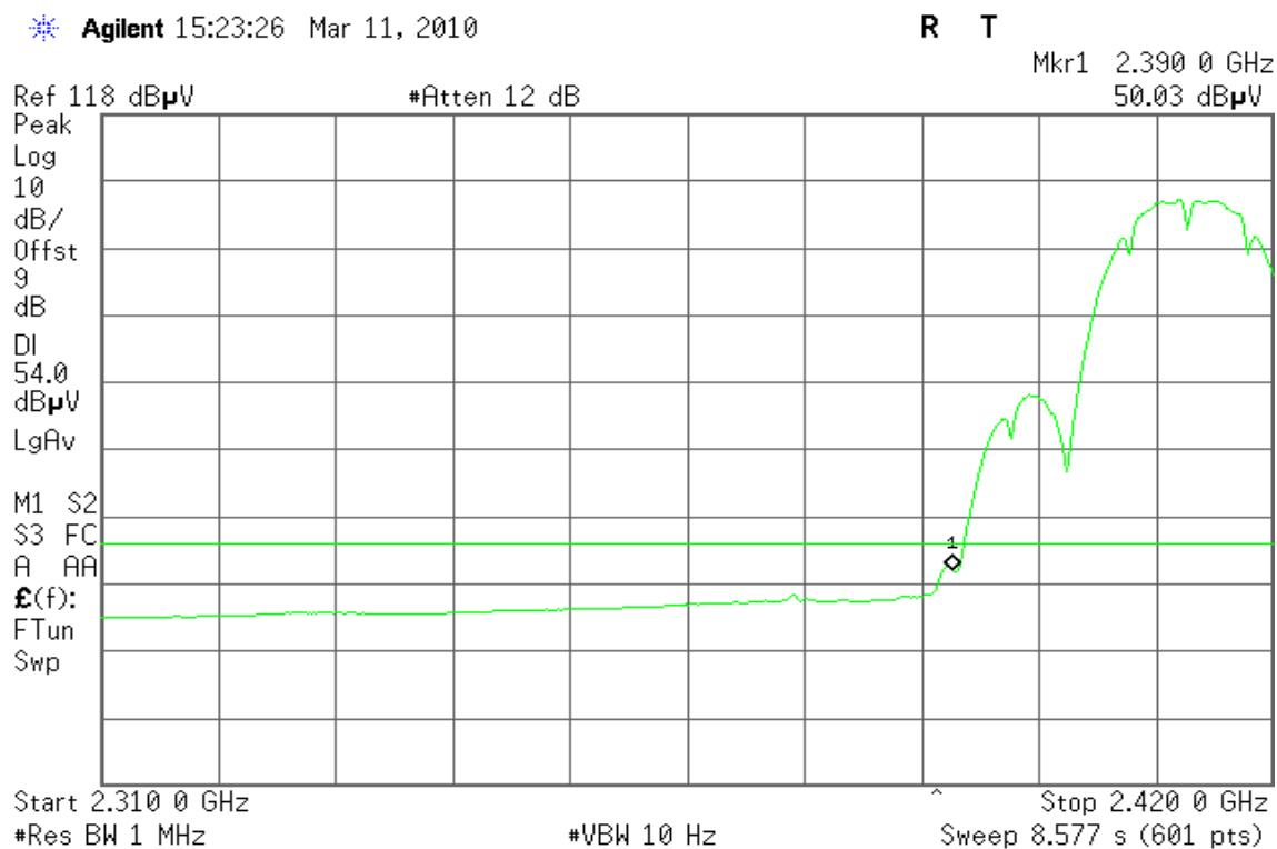
**Band Edges (IEEE 802.11b mode / CH High)****Detector mode: Peak****Polarity: Vertical**
