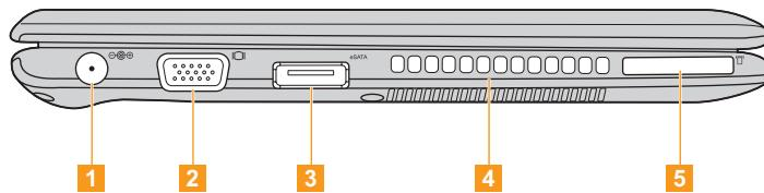
**1 AC power adapter jack** Connect the AC adapter here.
