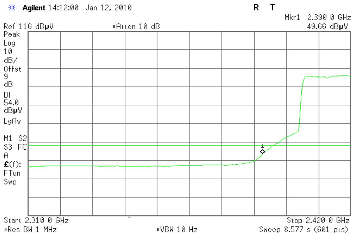
**Detector mode: Peak****Polarity: Horizontal**
