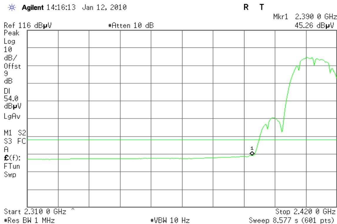
**Band Edges (IEEE 802.11b mode / CH High)****Detector mode: Peak****Polarity: Vertical**
