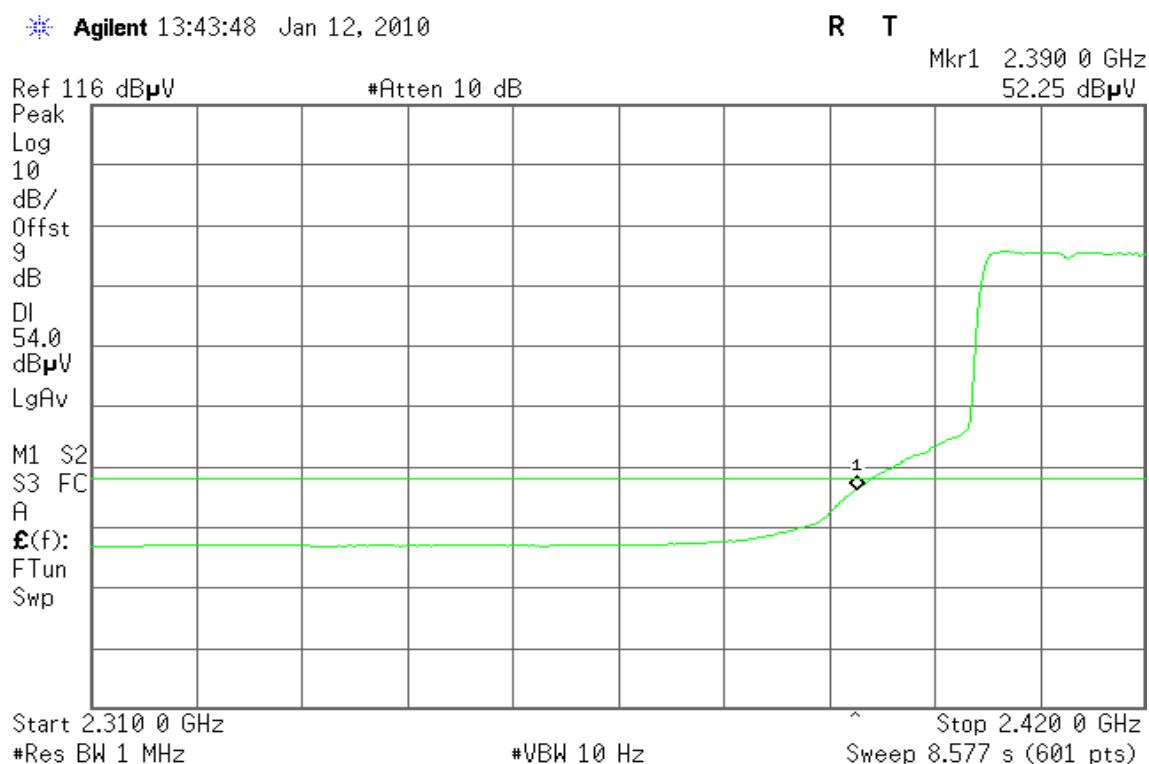
**Detector mode: Peak****Polarity: Horizontal**
