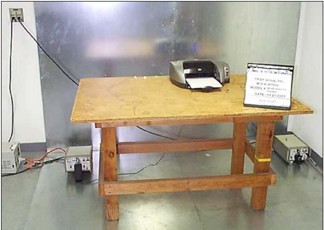
Mains Conducted Emissions - Front View Parallel
