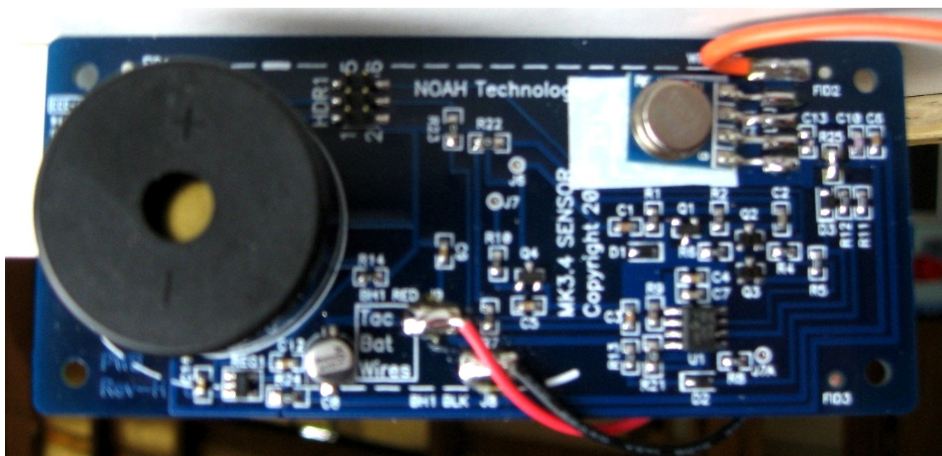
Sensor Circuit Board - Component Side With Antenna Moved Out of the Way
