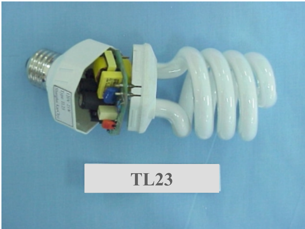
FIGURE 4 TWIST LAMP (M/N: TL23) COVER REMOVED
