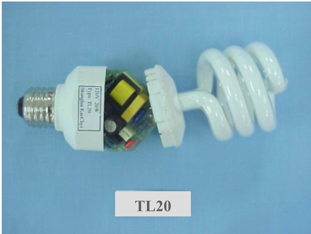
FIGURE 1 TWIST LAMP (M/N: TL20) COVER REMOVED
