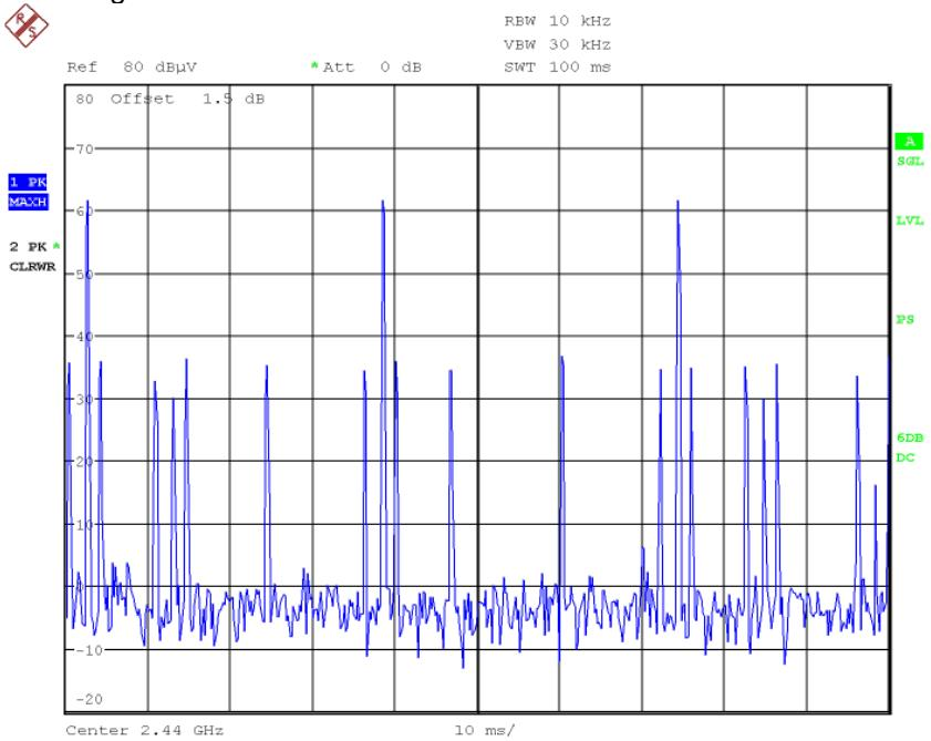
\* The smaller signals were from the other modules as a link was required between the modules to work correctly.
