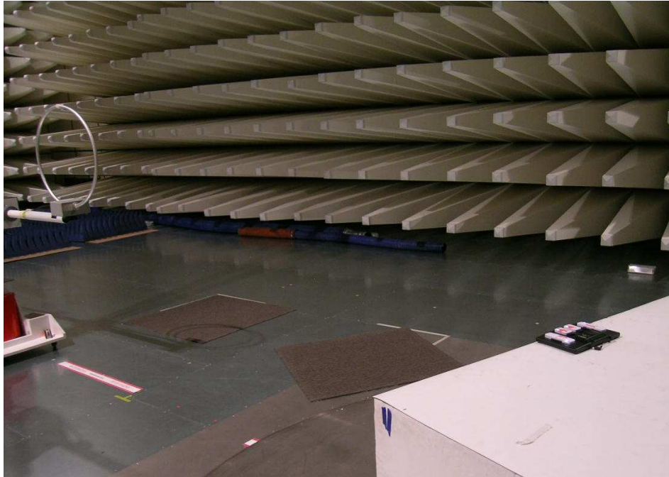
0.009MHz to 30MHz – Set-up with other devices (MD-E & RFD)
