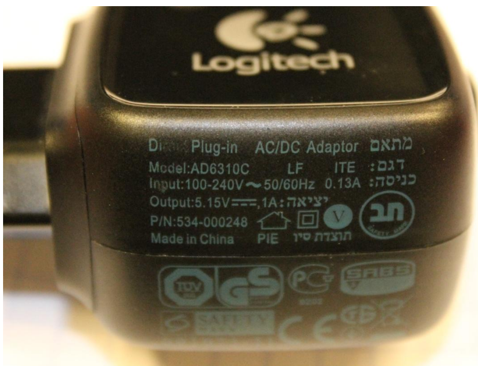
Photograph 4. AC/DC adaptor used in mains conducted emission test.
