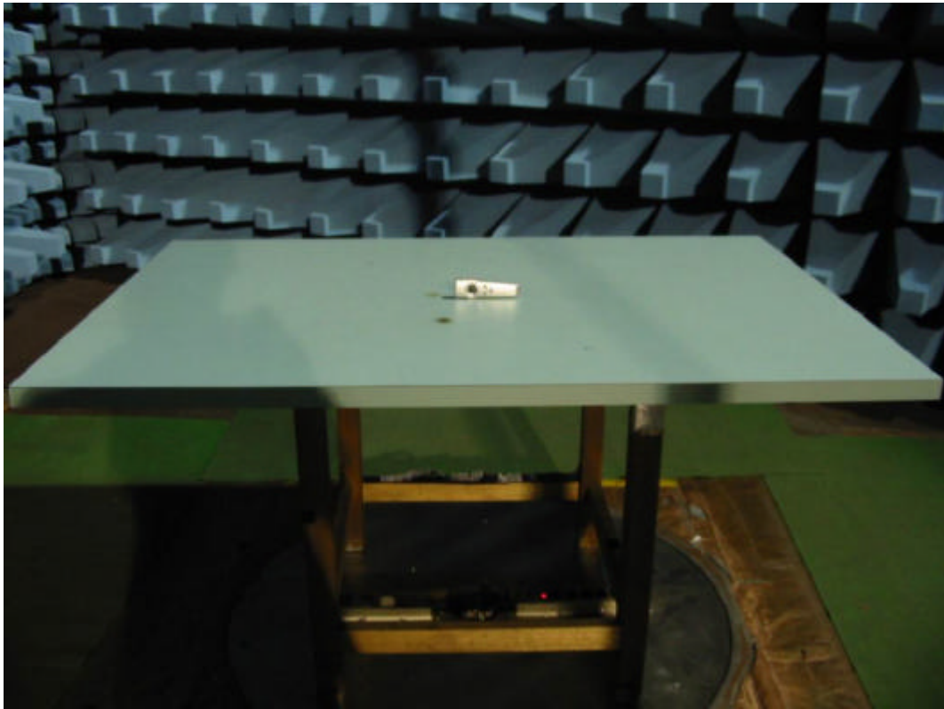
The Test Configuration of Z-axis
