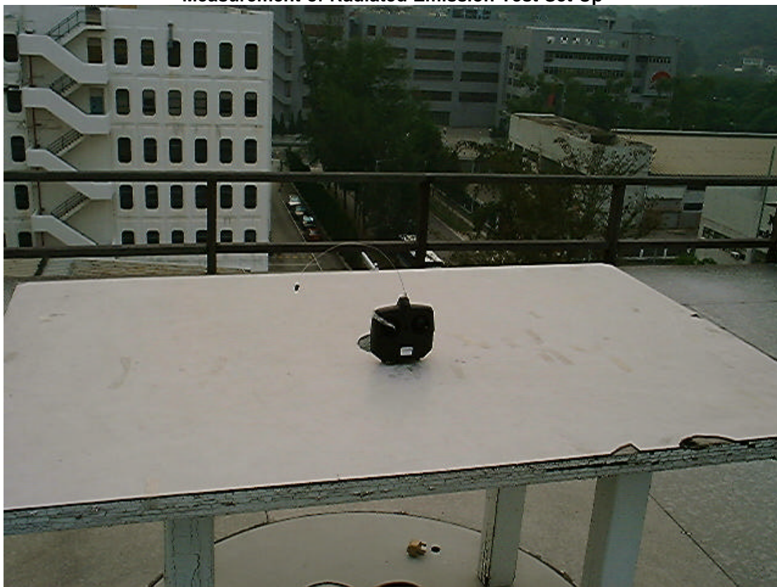
Measurement of Radiated Emission Test Set Up
