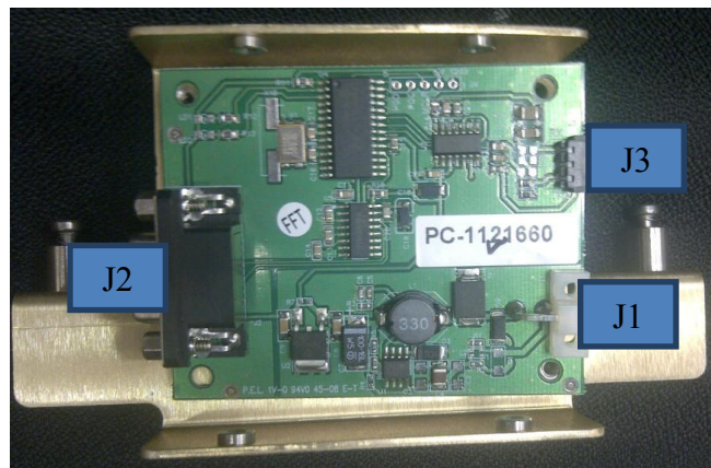
Figure 1 - LogiRead LT-LFS01-LM and an open representative metal housing
