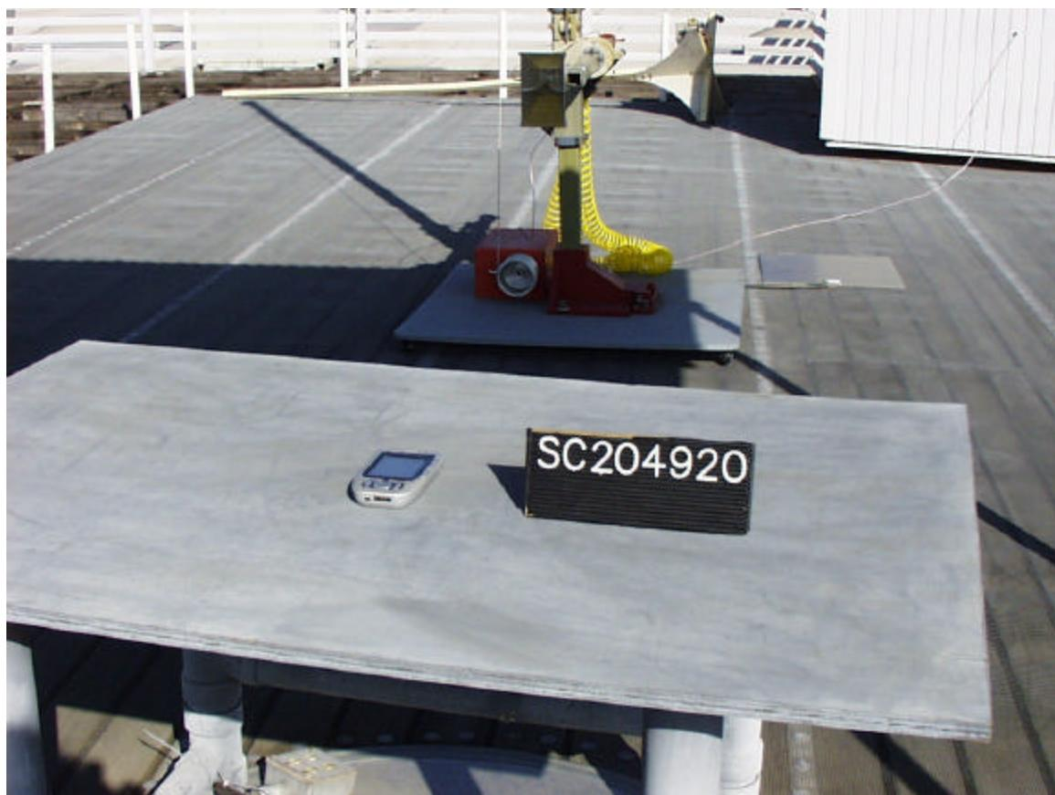
Test Setup for Bandwidth, Deactivation and Duty Cycle Measurements
