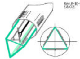
Figure 3.2 Triangular Probe Configuration
