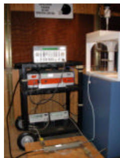
Figure 12.1 Dipole Validation Test Setup
