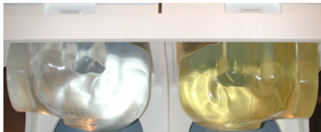
Figure 7.1 Left and Right SAM Phantom shells
