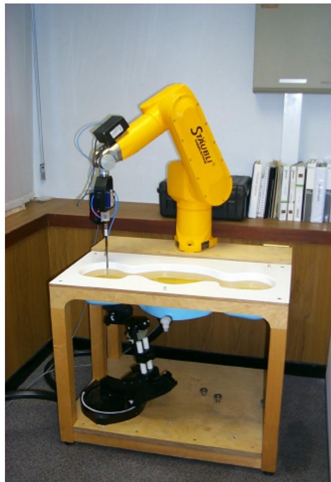
**Dasy 3 Measurement system****Figure 1.**
