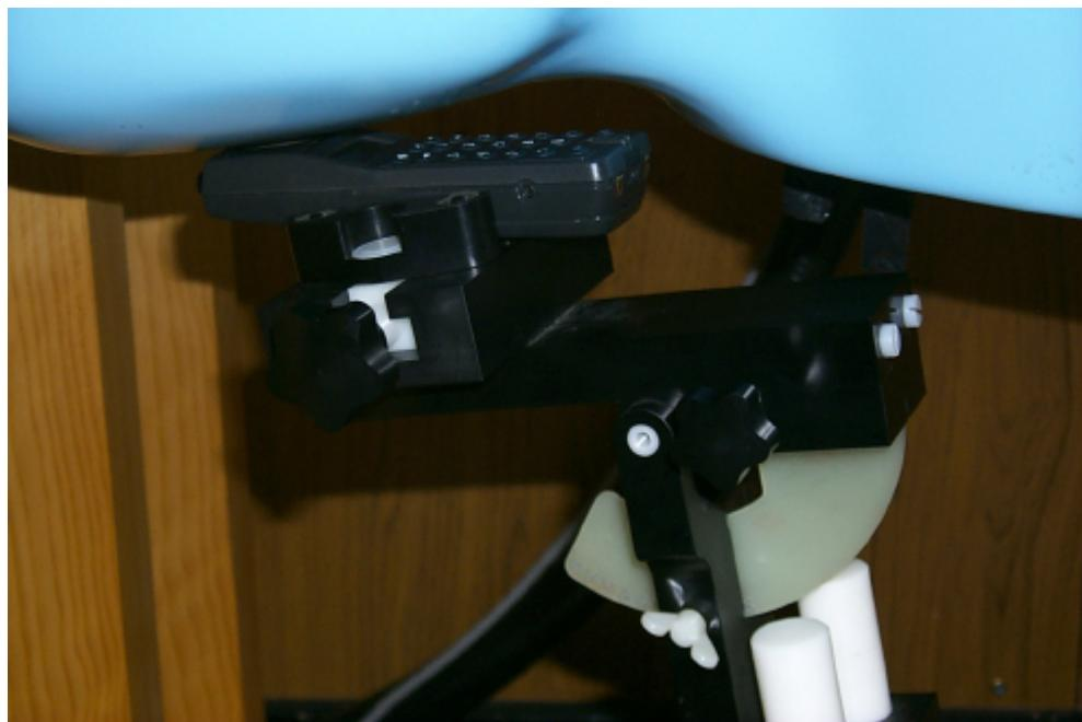
**Handset clamped into RH position**
