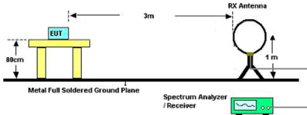
For Radiated Emissions: 30MHz~1GHz
