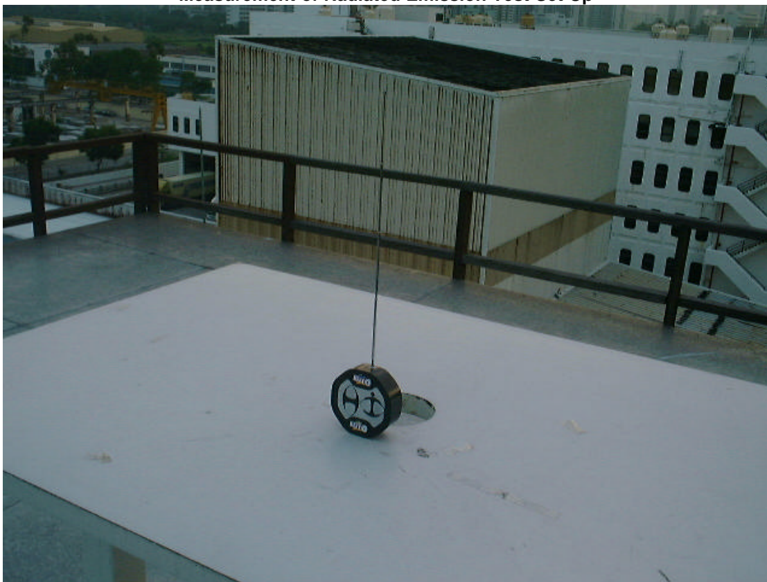
Measurement of Radiated Emission Test Set Up
