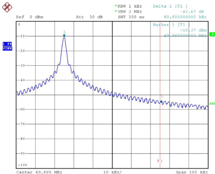
Bandedge Plot – Pursuant to FCC Part 15 Section 15. 235 Requirement (Pass)
