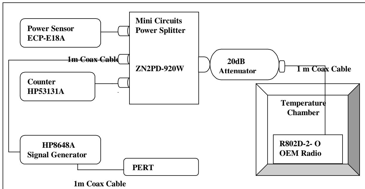
The chamber was switched on and the temperature was set to -30°C.
