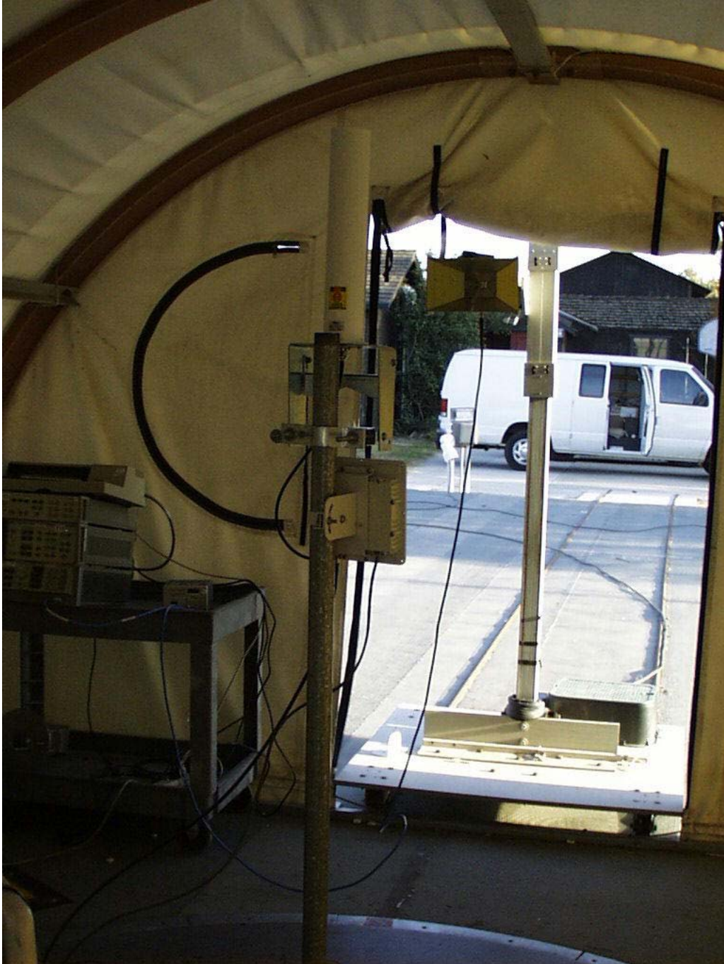
Radiated, sector antenna
