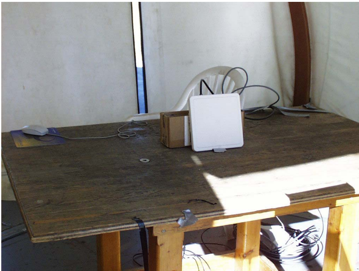
Subscriber unit with 18 dBi ntegral antenna, front view
