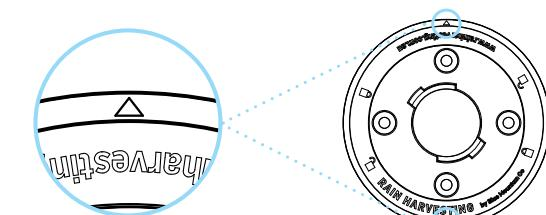
4. Screw the mounting plate to the top of the tank.
