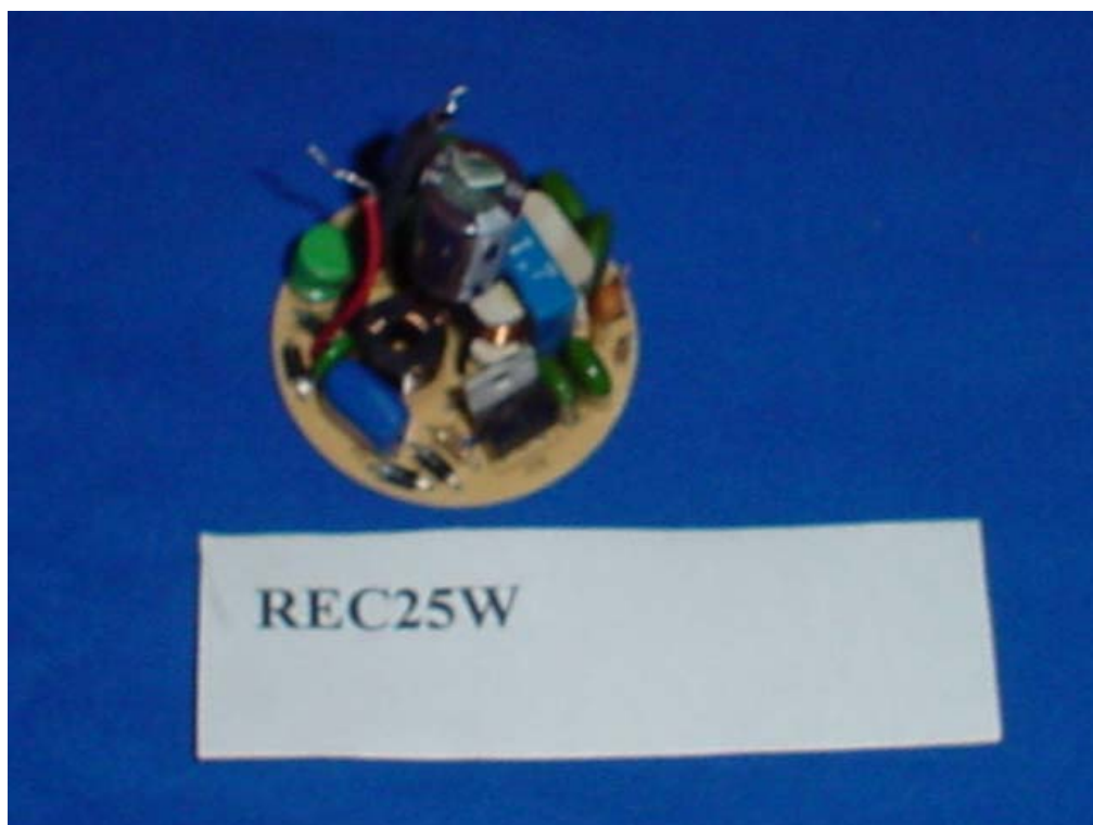
Figure 7 M/N: REC Series Main Board, Component Side
