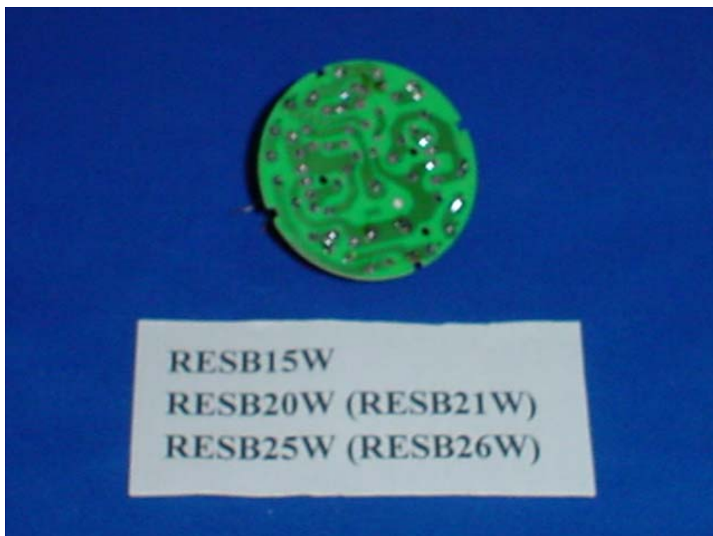
Figure 4 M/N: RESB Series Main Board, Soldered Side
