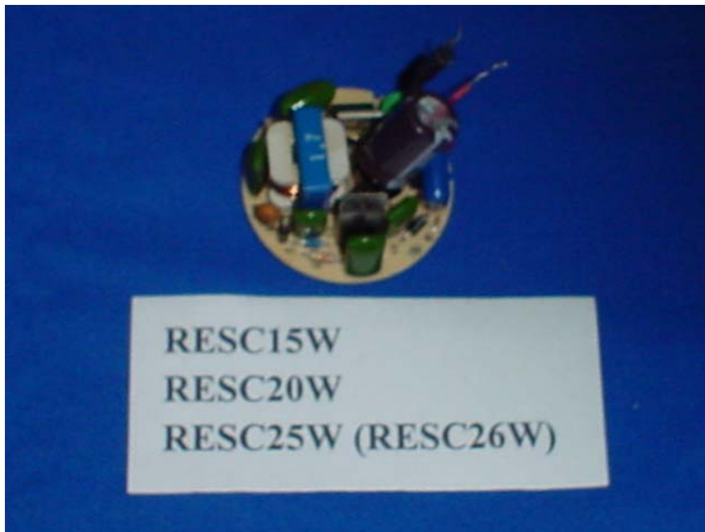
Figure 5 M/N: RESC Series Main Board, Component Side
