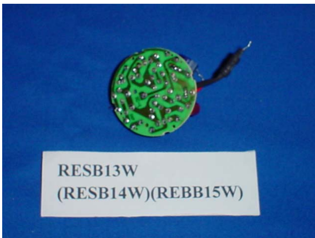
Figure 12 M/N: RESB 13W Main Board, Soldered Side
