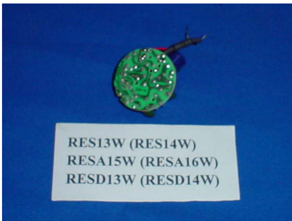
Figure 10 M/N: RES13W RESA15W RESD13W Main Board, Soldered Side
