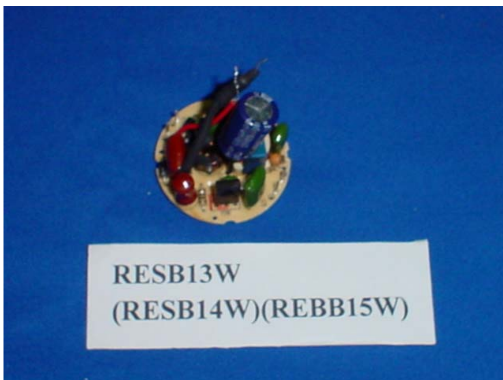
Figure 11 M/N: RESB 13W Main Board, Component Side
