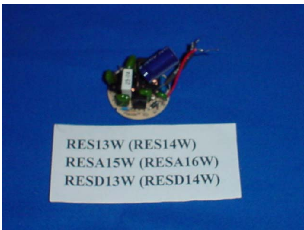
Figure 9 M/N: RES13W RESA15W RESD13W Main Board, Component Side
