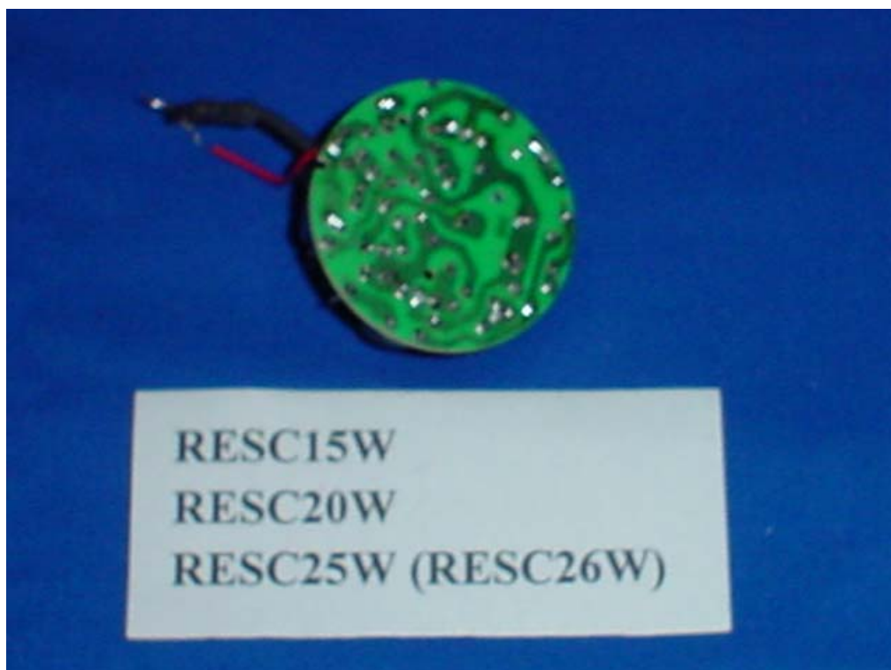
Figure 6 M/N: RESC Series Main Board, Soldered Side
