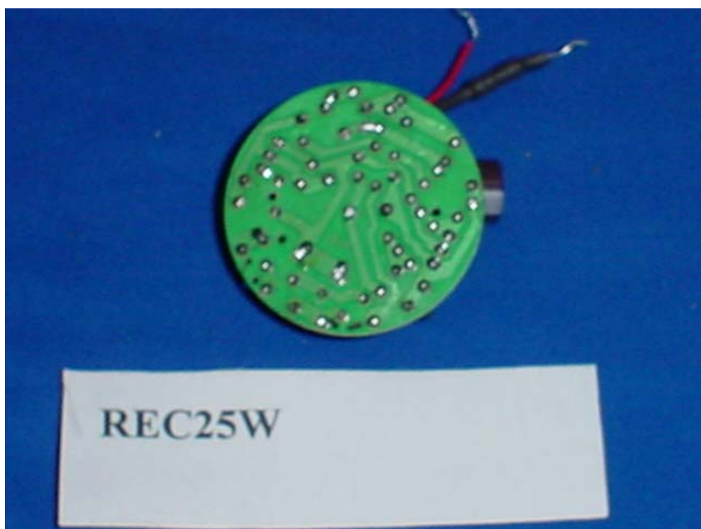
Figure 8 M/N: REC Series Main Board, Soldered Side
