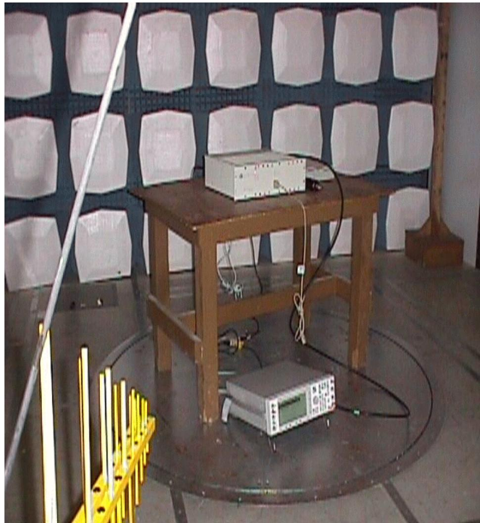
Photograph of Radiated Emissions Test Configuration
