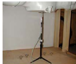
Figure 9.1 Dipole Verification Test Setup Diagram & Photo
