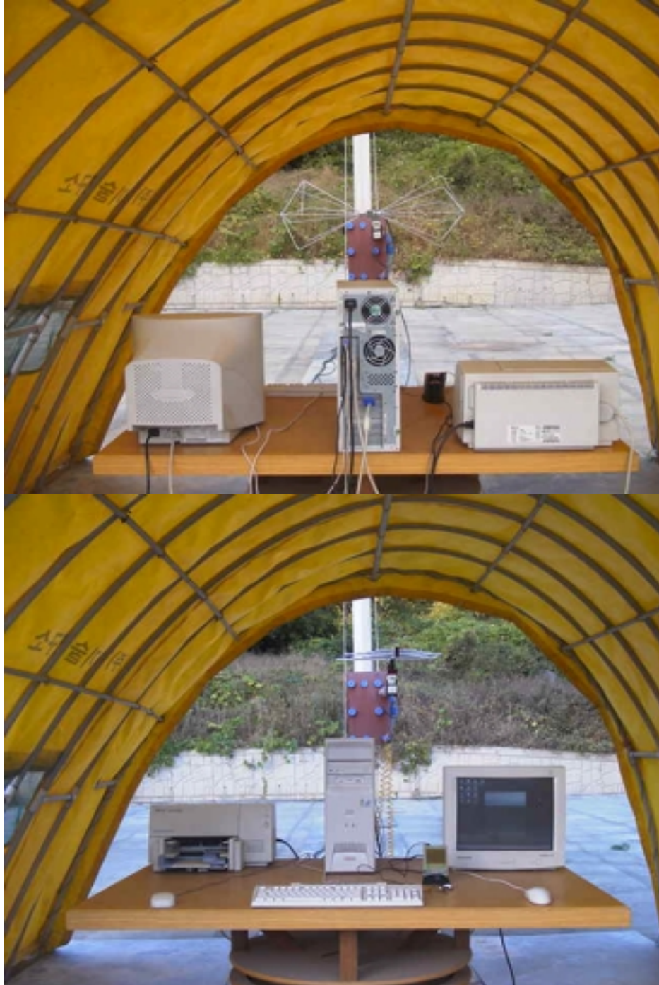
Photograph 1 : Setup for radiated Emissions
