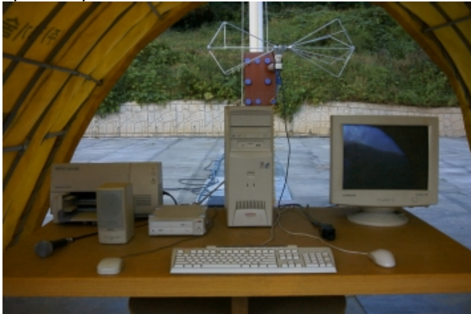
Photograph 1 : Setup for radiated Emissions
