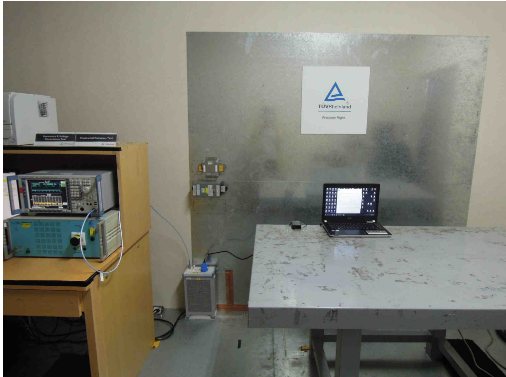
Photograph 6: Set-up for for Mains Conducted testing Front
