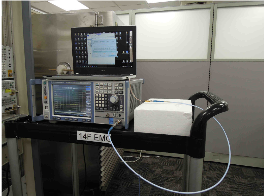
Photograph 4: Set-up for Conducted testing
